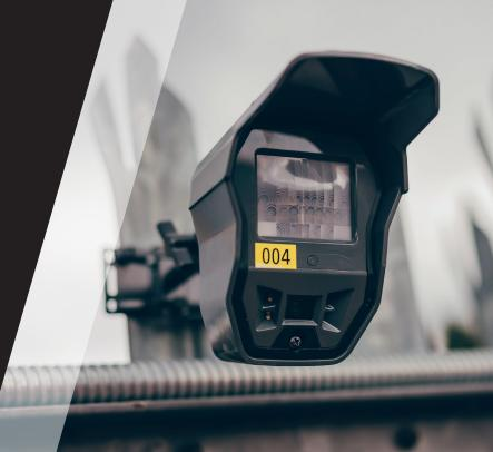
The RSI System is an external self sufficient intruder system with video verification. This rapid response system is a visible deterrent with the ability to work in harmony with other security solutions such as on site guards or mobile patrol.
